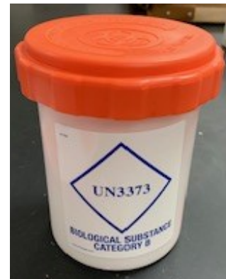
(3) Orange canister with appropriate marking that serves as RIGID OUTER PACKAGING.
