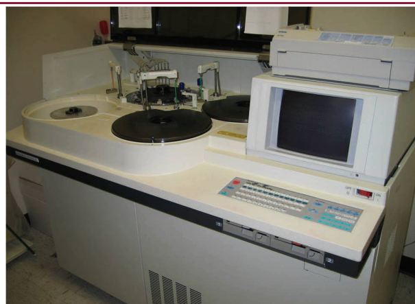
The Hitachi 717, an immunoassay analyzer, used for screening samples
