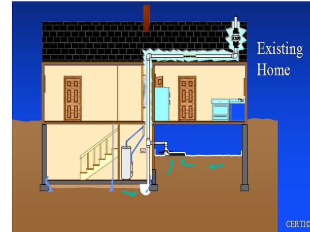
*A Step-By-Step Manual For Radon Reduction*
