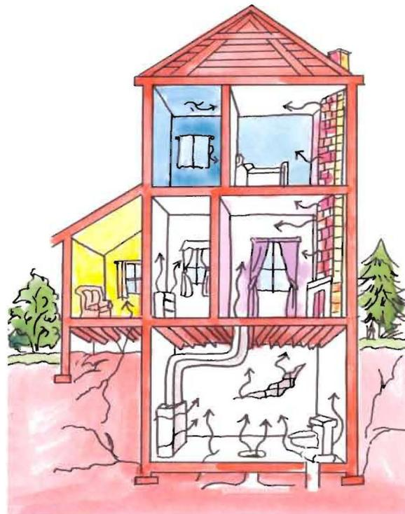
Radon enters your home from the soil under your home. Radon enters through every crack in your foundation and where electrical, plumbing and other pipes/fixtures penetrate your foundation. Radon even enters where the walls and floors join.
